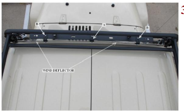
GOBI JEEP JK STEALTH BAR WIND DEFLECTOR INSTALLED CORRECTLY IN A CURVED POSITION. CENTER BRACKET (A) POSITIONED FULLY FORWARD AND BOTH END BRACKETS (B) POSITIONED TOWARDS THE REAR FORMING A CURVE IN THE WIND DEFLECTOR TO PREVENT VIBRATION DURING HIGH SPEED DRIVING.
