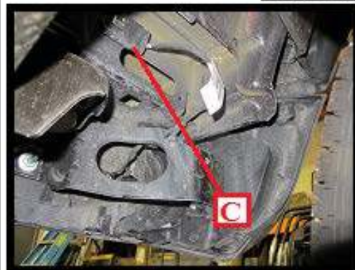
Just above the rear splash guard support bracket you will find the rear bumper sensor connection (C) shown above
