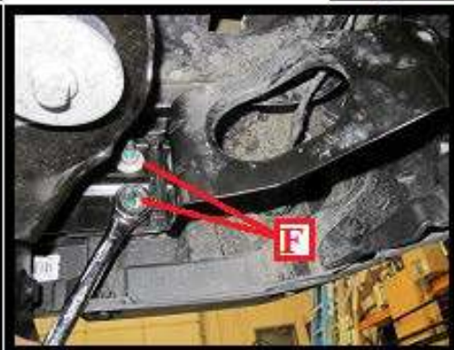
Remove 2 nuts (F) shown above both driver and passenger sides using a 16mm socket or box end wrench
