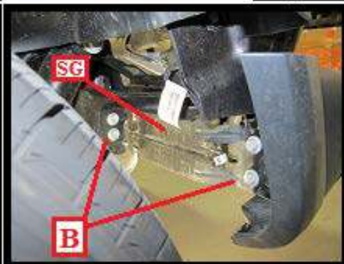
Remove splash guard support bracket (SG) by removing 4 screws (B) as shown above using a 16mm socket
