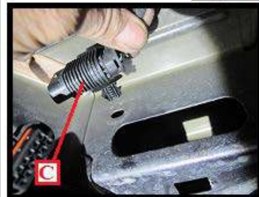
Pull out sensor connection (C) anchored to body as shown above and allow to hang freely
