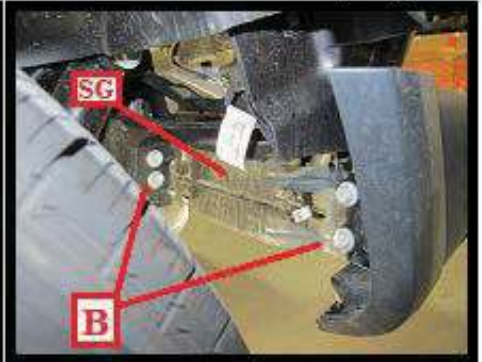
Remove splash guard support bracket (SG) by removing 4 screws (B) as shown above using a 16mm socket
