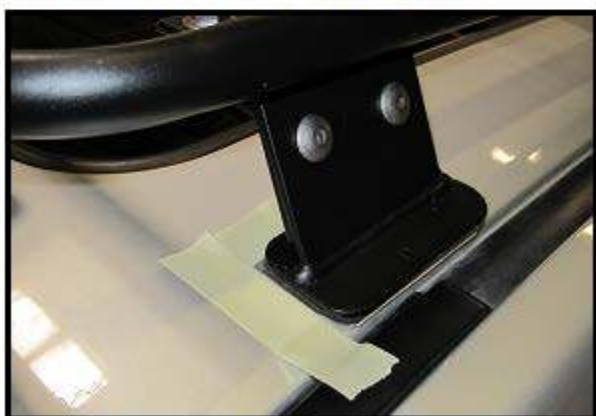
Fig. 18 Position both front driver and passenger side brackets as shown above and center roof rack on vehicle as shown in Fig. 19. Place masking tape as shown around the inside and front edges of support bracket.
