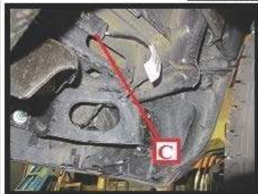
Just above the rear splash guard support bracket you will find the rear bumper sensor connection (C) shown above
